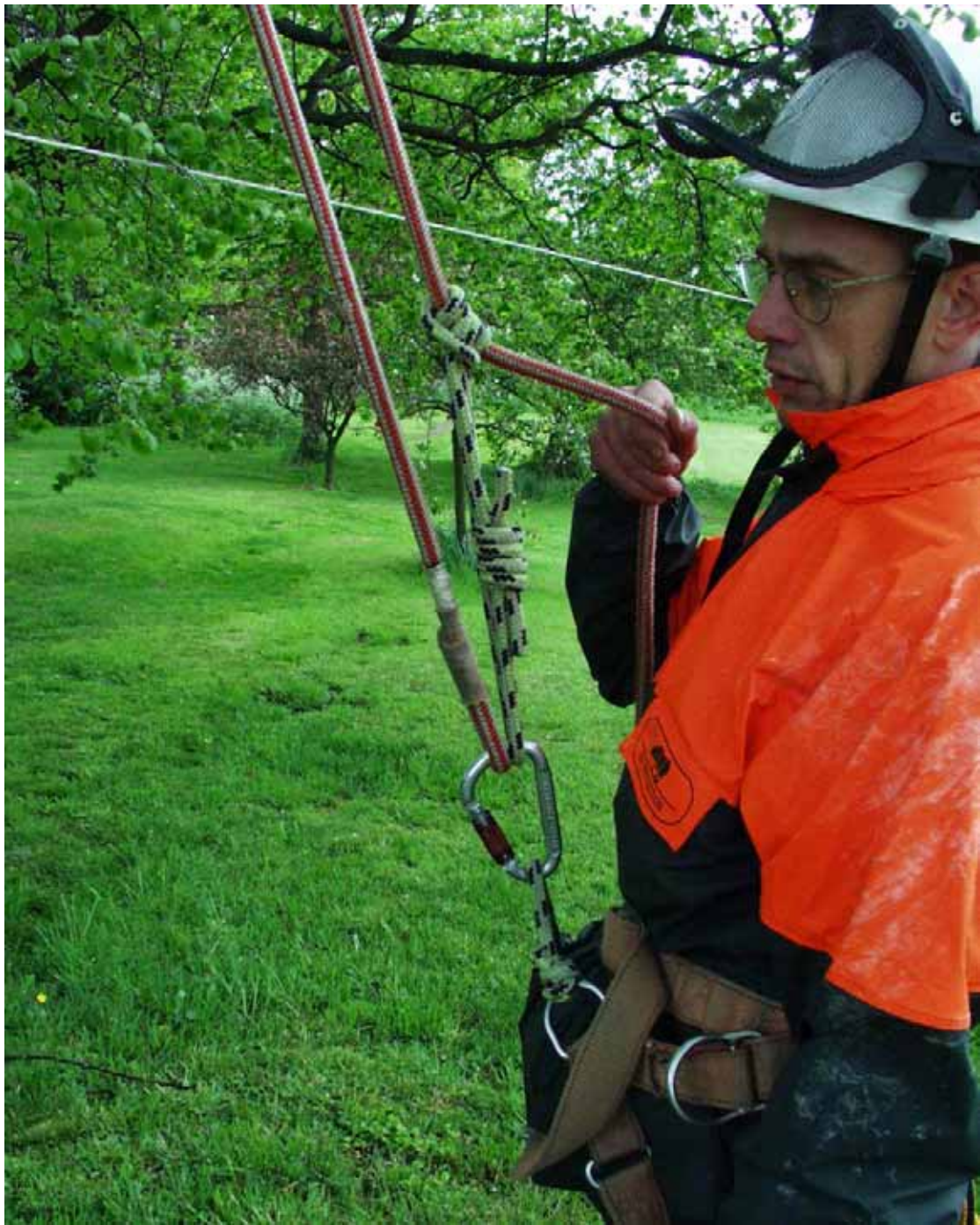
Figure 1 – Basic configuration of climbing and prussik ropes.
